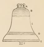
The various parts of the bells are A, the Canons; B, the Shoulder; c, the Waist; the thick part between D and E, the Sound Bow; E, the Rim or lip; F, the Clapper.
